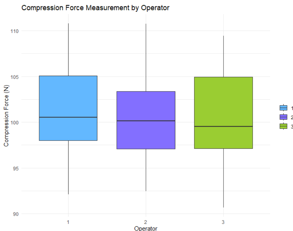
Figure 20: Spring measurements box plots grouped by operator.
