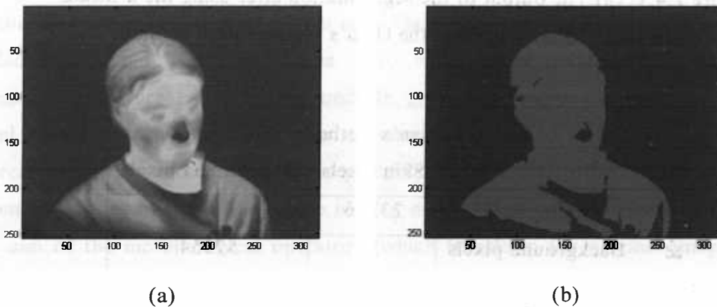
Figure 2.3.2.2: (a) The input image and (b) the image after applying Otsu's algorithm
